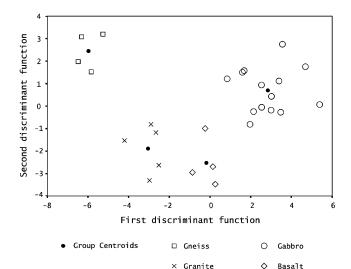
FIG. 7. Plot of samples in data set B in the space formed by the first and second discriminant functions. The cases are labeled by the true lithotype.
