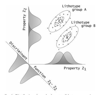
FIG. 1. Distribution of samples from two lithotype groups in a space of two physical properties  $z_1$  and  $z_2$ . The marginal probability densities for each group are represented near to the axes, showing significant overlap between the groups for both  $z_1$  and  $z_2$ . The group separation is improved for the discriminant function  $z_1 - z_2$ . Among all possible linear combinations of the original variables, this particular combination optimizes the group separation.
